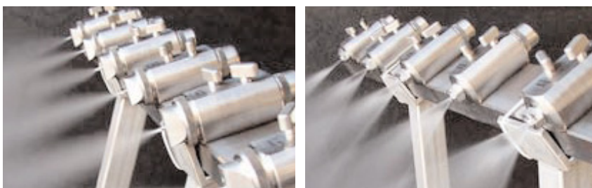
The need to change fewer components means that the two-substance nozzles used for film coating (left) can be converted to pressure nozzles (right) for sugar coating.
